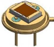
1. **CLEANING:** Clean outside edge of header and cap if applicable with a 50/50 mixture of isopropyl alcohol and water. Use light strokes with a cotton tipped applicator. Avoid getting mixture inside of housing. Do not touch lead wires or surface of detector. Do not use acetone or halogenated solvents.
